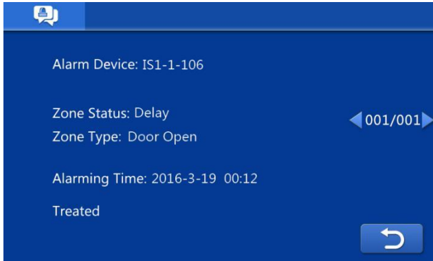
Alarm interface of door opened too long
